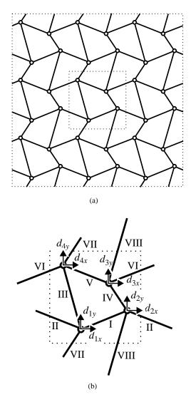
Fig. 4. (a) A perturbed square grid structure, showing a possible unit cell and (b) a possible numbering scheme for bar extensions (I–VIII) and displacements of nodes  $(d_{1x}-d_{4y})$  in the unit cell.
