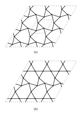
Fig. 5. Two mechanisms of the kagome structure: (a) the finite mechanism; and (b) one possible infinitesimal mechanism.
