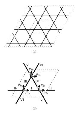
Fig. 3. (a) The kagome structure, showing a possible unit cell and (b) a possible numbering scheme for bar forces (I–VI) and applied loads  $(p_{1x}-p_{3y})$  in the unit cell.
