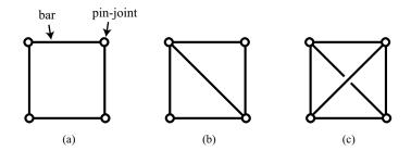
Fig. 1. (a) A *kinematically indeterminate* structure, with one mechanism, (b) a *statically and kinematically determinate* structure and (c) a *statically indeterminate* structure, with one state of self-stress.
