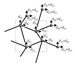
Fig. 7. An augmented nodal displacement numbering scheme for the perturbed square grid, allowing displacements of the nodes  $(d_{1x}-d_{4y})$  and deformation of the unit cell  $(d_{xx}, d_{yy}, d_{xy})$ .
